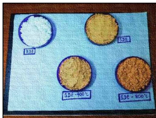
Figure 2. The differences of the colour in four types of adsorbents: (a) RDE (b) SDE (c) SDE-400 °C and (d) SDE-800 °C
